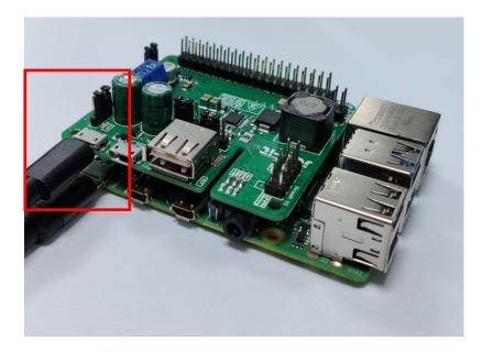
Your StromPi is in flash mode when the blue LED lights up dimly, as shown in the picture below
