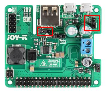
Now put your StromPi on your Raspberry Pi and supply both with power via the micro-USB port (or USB-C).
