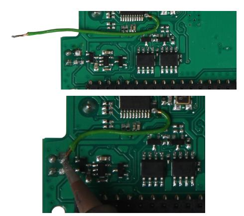
Finally the other end of the cable is soldered to the lower solder pad.
