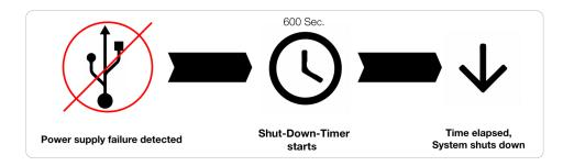
If the StromPi 3 now detects a power failure, the timer starts. After 10 minutes the StromPi 3 will then disconnect the power supply to the Raspberry Pi. Additionally we provide a script that can detect a power failure either via the serial console or via a GPIO pin and then shut down the Raspberry Pi safely. The shutdown timer can be set in the config script by **Shutdown Timer**.
