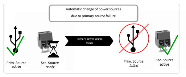
In total there are six different modes possible. The primary power source is the main power source. The secondary power source will take over when the primary source fails.
