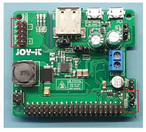
In revision 1.1 the modifications, which had to be soldered in revision 1, have been incorporated into the PCB design. This means that **soldering is no longer necessary** for the PowerOn button function and for the serialless function.
