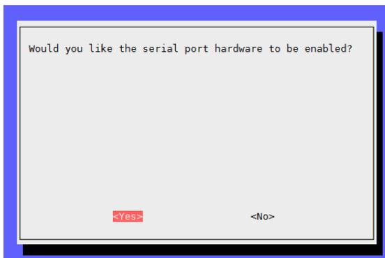
After confirming again, you can exit the menu with **Finish**. Answer the question after restarting the device with **Yes**. The serial interface is now activated and the serial console deactivated.
