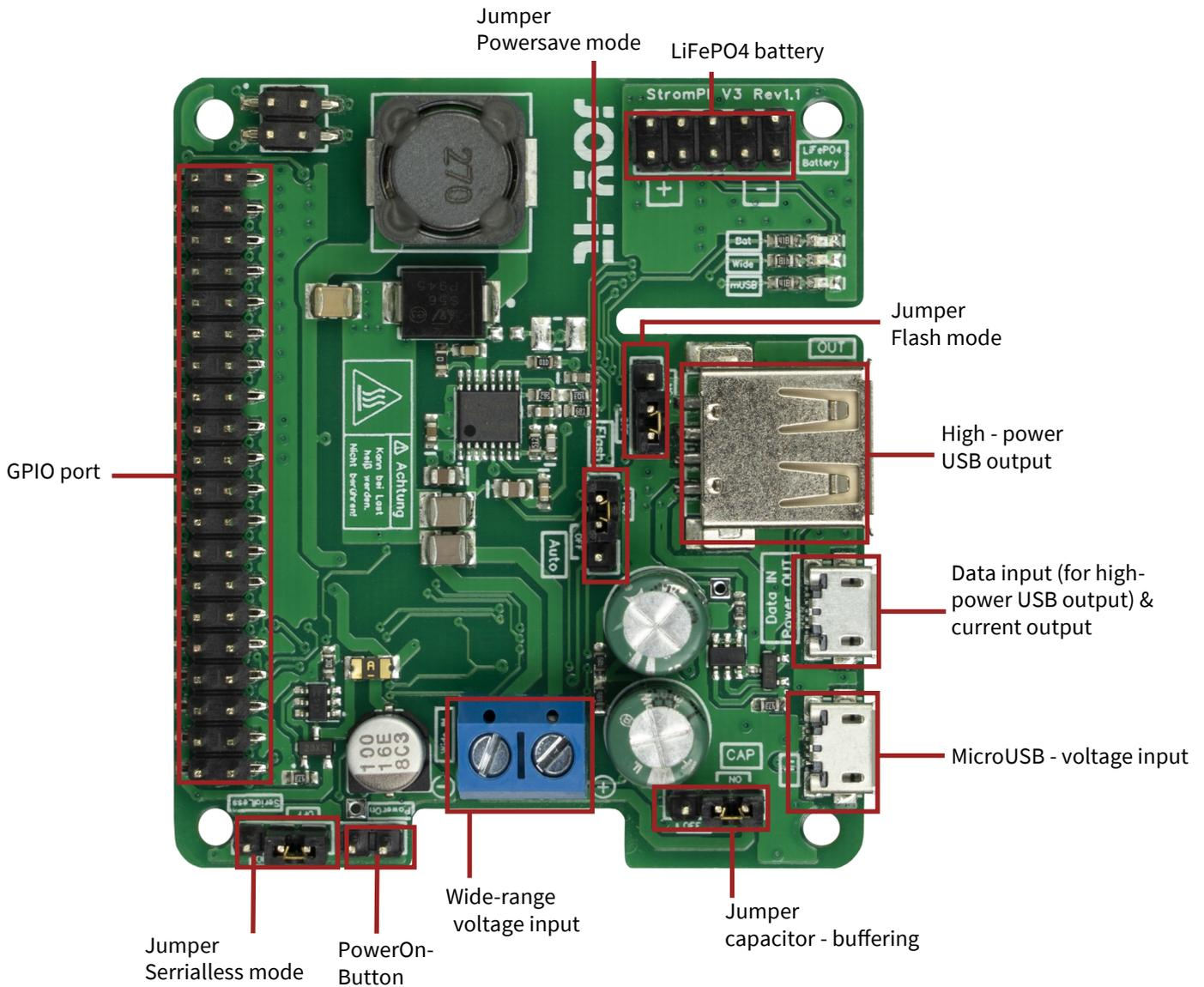
The newly added serialless jumper connects the GPIO 21 (pin 40) of the Raspberry Pi to a GPIO of the microcontroller when set to "ON". The serialless function must still be activated as usual in the configuration of the StromPi 3.
