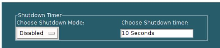
To activate the Shutdown Timer, select **Enable** at **Choose Shutdown Mode** and enter the desired shutdown time in seconds into the adjacent field. Finally, confirm with Update.
