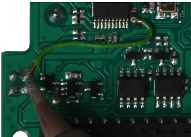
Finally the other end of the cable is soldered to the lower solder pad.
