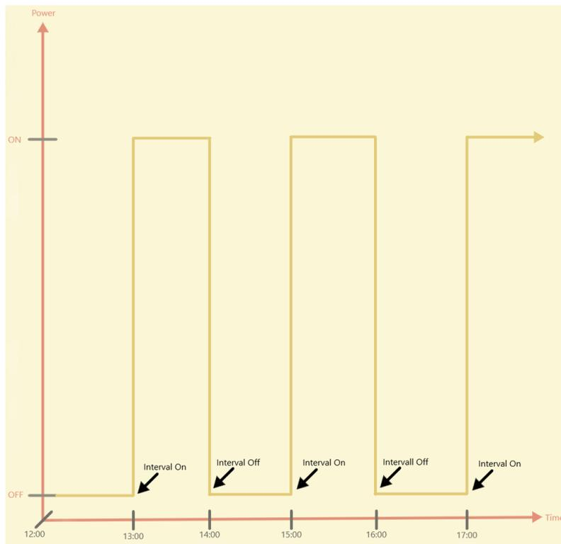
The interval function allows you to define time intervals in which the Raspberry Pi is switched off and on again with the help of the StromPi 3. You can activate and configure this function in the config script by **Timer**.
