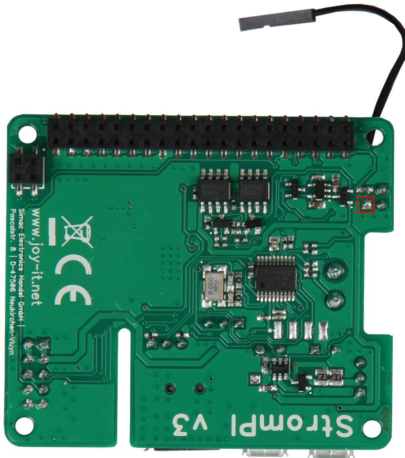
The other end of the cable is connected to a free GPIO pin.
