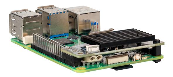
The microcontroller installed on the board reads the status of the button. If the button is held down for one second during operation, the GPIO4 of the Raspberry Pi is pulled low and 10 seconds later the voltage converter is switched off.
