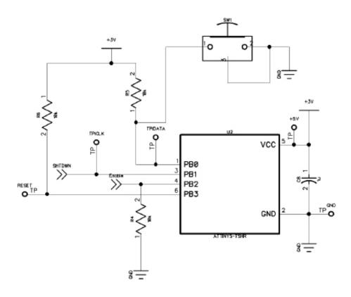
SHTDWN is the connection to the GPIO4 of the Raspberry Pi. Enable is the connection to the enable pin of the voltage converter on the board.
